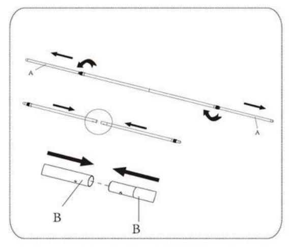
To connect B-B, pull out pole A to the tlimited stop then tighten the plastic bolt. Same way to the pole #C-D.
