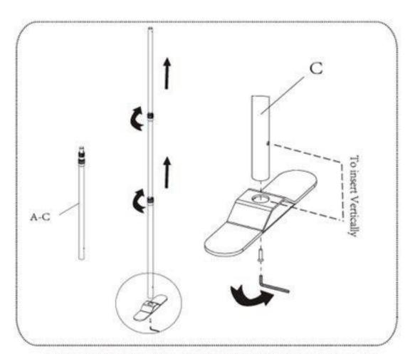
To insert pole #A-C into the socket of base vertically then (2) tightening; Afterwards, screw off #A-C to the limited stop and screw up the plastic bolt.
